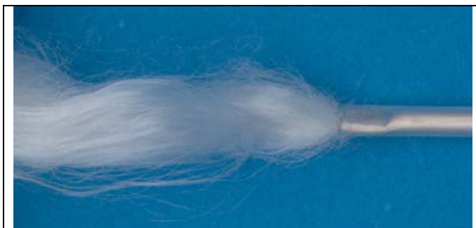
Figure 1. Close-up of the FiberSecure, a tow (unbraided bundle) of twelve-micron polyester fibers, converging into the heel of a needle.
